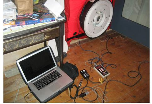
then used to obtain data to apportion the measured leakage between the new construction (addition/rebuild) and retrofit portions of the project. The older portion of the building measured at 348 CFM @50 Pa (0.8 ACH 50 and 0.06 CFM per square foot of enclosure) and the new construction addition measured 125 CFM @50 Pa (0.9 ACH 50 and 0.06 CFM per square foot of enclosure).
