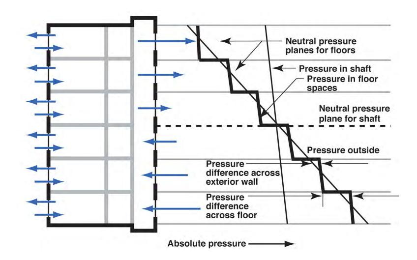
Figure 11.9: Multi-storey building with floor spaces isolated from vertical shafts (Adapted from G.O. Handegord, 1998)
