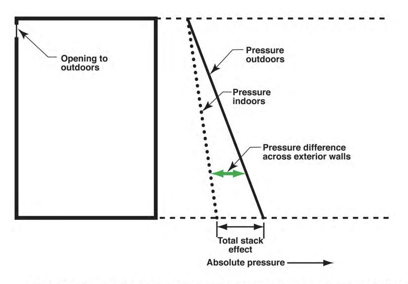
Figure 11.2: Building with no internal separations with opening at the top (Adapted from G.O. Handegord, 1998)
