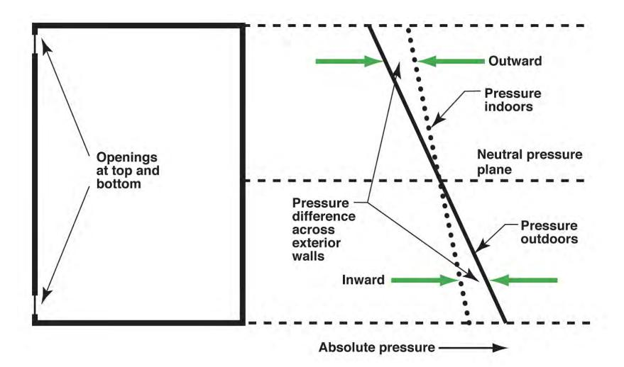
Figure 11.3: Building with no internal separations with openings at top and bottom (Adapted from G.O. Handegord, 1998)
