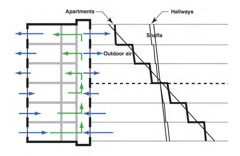
Figure 11.12: Apartment building with tighter apartment entry doors (Adapted from G.O. Handegord, 1998)
