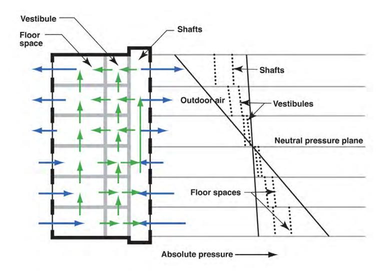
Figure 11.8: Stack effect pressures in high rise office building (Adapted from G.O. Handegord, 1998)
