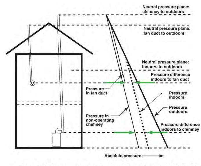
Figure 11.5: Two storey house with non-operating chimney and exhaust fan (Adapted from G.O. Handegord, 1998)
