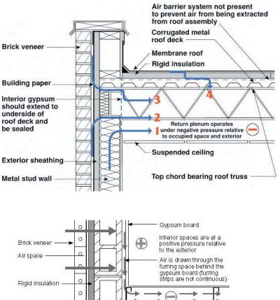
Cavity spaces within the demising wall are at a negative pressure relative
