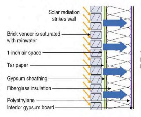
Vapor is driven inward by a high vapor pressure differential between the cavity and the interior
