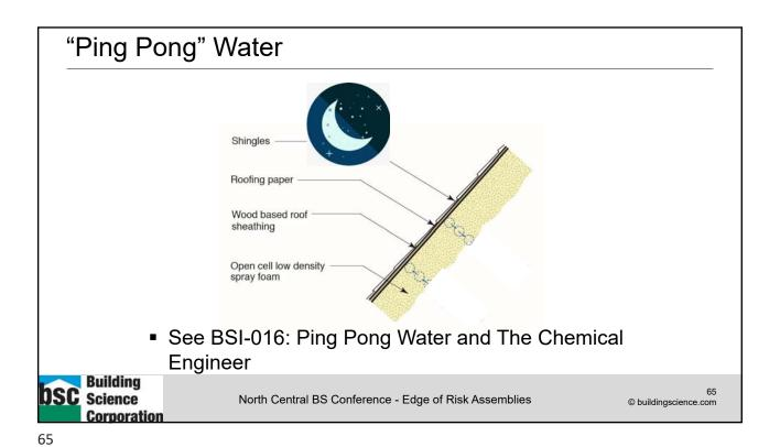
"Ping Pong" Water Shingles Roofing paper Wood based roof sheathing Open cell low density Each "Ping" and "Pong" spray foam bounces the water molecules up the slope "Gas separation process similar to pressure swing adsorption" Solar-powered moisture concentration machine Building **SC** Science North Central BS Conference - Edge of Risk Assemblies © buildingscience.com Corporation
