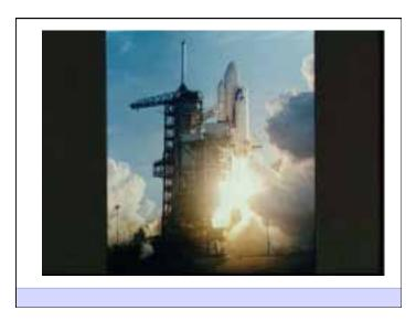
Early Shuttle Fights Had Aluminum Paint Over External Tank Foam - Note White Color On Tank - Aluminum Paint Removed To Save Weight
