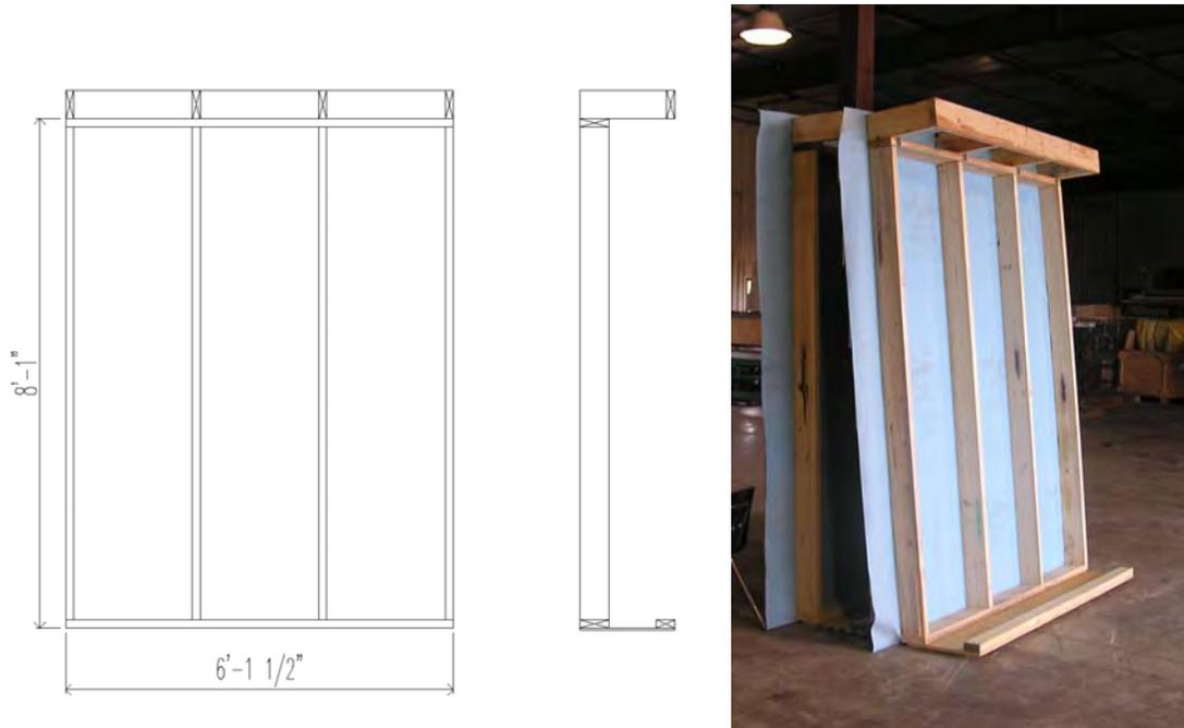
**Figure 1: Test Panel Configuration**
