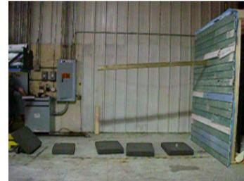
Stud penetrated cladding but not through Wall 2
