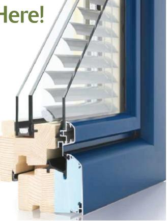
Figure 1. A composite foam and wood frame with aluminum cladding, and integrated operable shading (Courtesy Holz & Form Canada).
