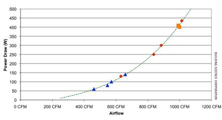
Figure 1. The figure demonstrates that the horsepower varies with the cube of the RPM (and therefore the cube of the CFM).
