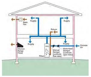
Ventilation System 3: Central Fan-Integrated Supply (CFIS) Ventilation
