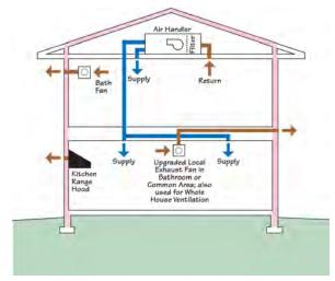
Ventilation System 4a: Exhaust-only single point ventilation system
