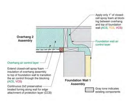
Foundation Wall 1 to Overhanging Floor 2 at Inside Corner
