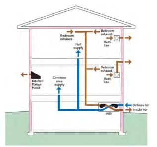
Ventilation System 1a: balanced heat recovery ventilation system with dedicated ductwork and ventilation air returns located in bedrooms
