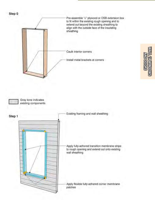
Flanged Window with Extension Box in Wall 1A—Installation Sequence
