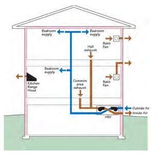
Ventilation System 1b: balanced heat recovery ventilation system with dedicated ductwork and ventilation supplies located in bedrooms
