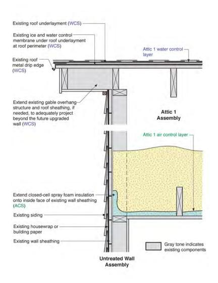
Attic 1 to Untreated Wall-Rake
