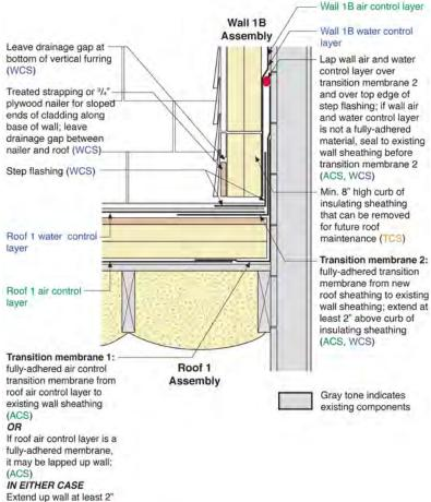
Extend up wall at least 2" above step flashing (ACS)
