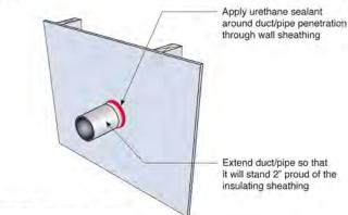
Duct/Pipe Penetration Through Wall 1A-Installation Sequence
