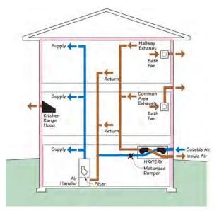
Ventilation System 2b: balanced heat recovery ventilation semi-integrated with forced-air heating and cooling supply distribution ductwork
