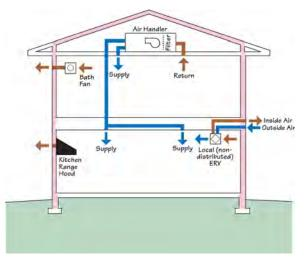
Ventilation System 4b: Non-distributed heat recovery ventilation system
