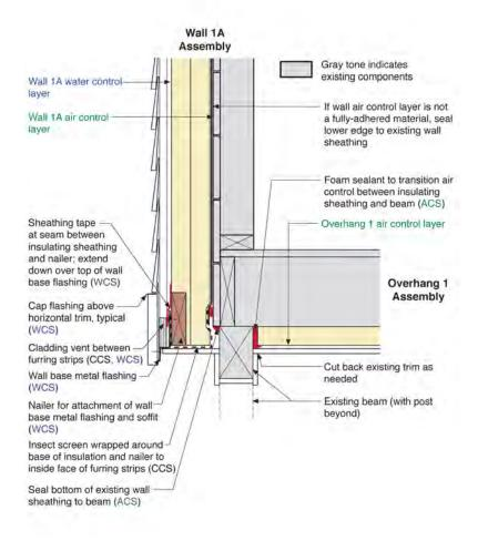
Wall 1A to Overhanging Floor 1 with Beam at Outside Corner
