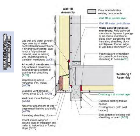
Wall 1B to Overhanging Floor 1 with Beam at Outside Corner
