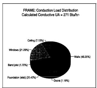
**Figure la.** Conduction Heating Load Distribution and Calculated Conductive UA for the Stud-Frame House
