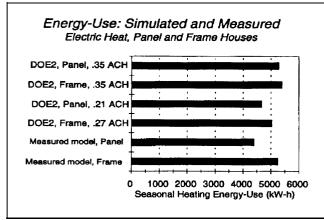
**Figure 3.** Heating Energy-Use by Measured Data Regression Model and Hourly Simulation Using TMY Weather Data for Two Air Change Rates
