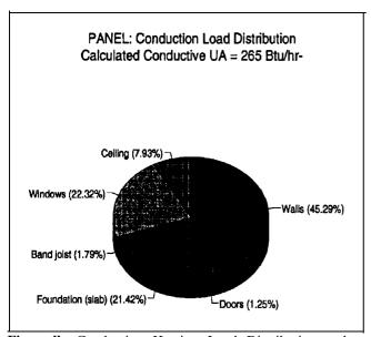
**Figure lb.** Conduction Heating Load Distribution and Calculated Conductive UA for the SSIC Panel House
