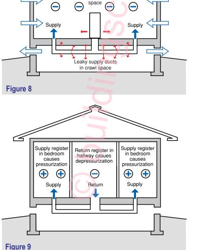
moisture removal capability of the cooling system is unable to remove this moisture, mold and other biological growth also occurs.
