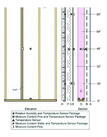
Figure 3 Typical wall setup and sensor layout for full-scale wall testing in Waterloo, ON.
