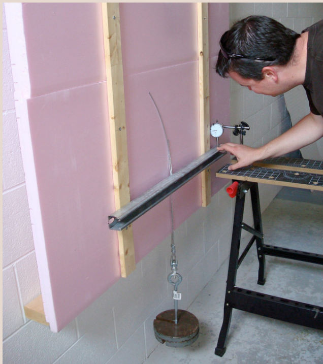
Photograph 3: Bench Top Testing —Screws experience mostly “shear” and not “moment” (bending) loads because the screws can’t rotate into the foam due to the compressive strength of the foam pushing back against the 1x4 wood furring.
