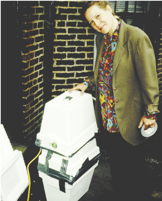
Photograph 4: Portable Site Constructed Environmental Chamber —Duct tape holds together some foam coolers containing a light bulb attached to an extension cord. Disassembled cabinetry is placed inside the chamber and heated to the operating temperature of the cabinets.
