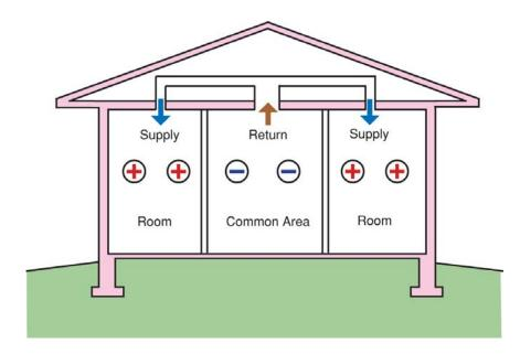
Figure 2: Pressure Effect Due to Unbalanced Air Flows
