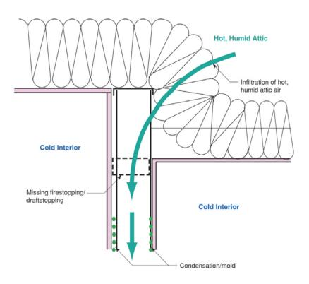
Figure 3: Air Pressure Effects within Building Cavities
