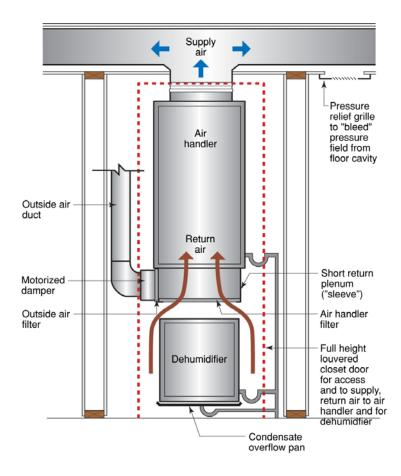
Figure 6: Air Handler Schematic with Stand-Alone Dehumidifier
