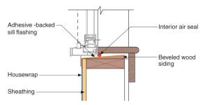
A piece of wood bevel siding nailed over the sill to create positive drainage toward the exterior is even better. Note that the rough opening needs to be enlarged to account for this and tapered shims in the opposite direction of the slope may be required.
