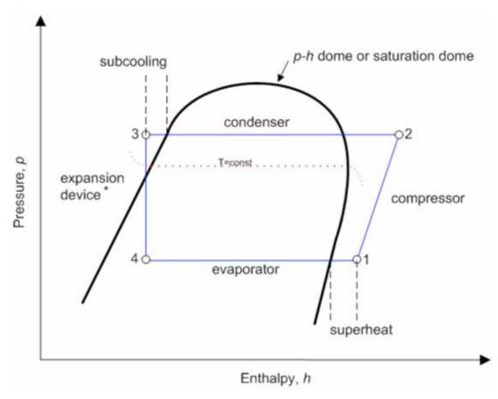
*Figure 2*: Vapor Compression System Pressure vs. Enthalpy
