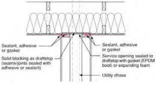
Flexible gasket sealed to top plate or other solid blocking allows movement of penetrating element without losing the air seal Recessed ceiling fixtures in insulated ceiling should be both insulation contact ("IC")- and air tight rated. The housing of the recessed fixture should also be sealed (with caulk or an effective gasket) to the ceiling gypsum board.
