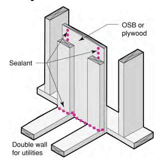
Solid draftstop material sealed to framing to isolate utility chase cavity
