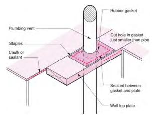
Flexible gasket sealed to top plate or other solid blocking allows movement of penetrating element without losing the air seal
