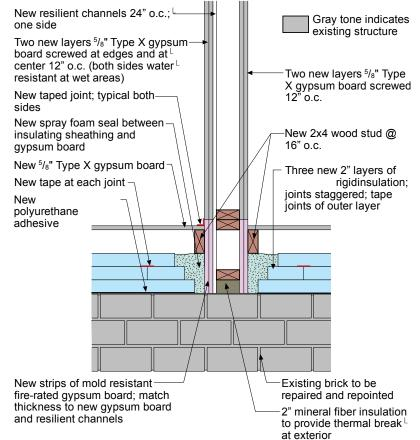
Figure 11: Rated partition intersection with exterior wall
