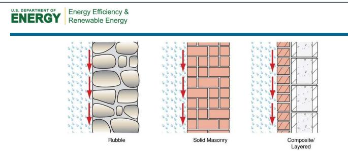
Figure 4: Examples of mass masonry walls and rain control
