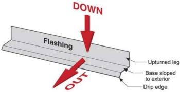
Figure 3: The "down" and "out" approach to flashing
