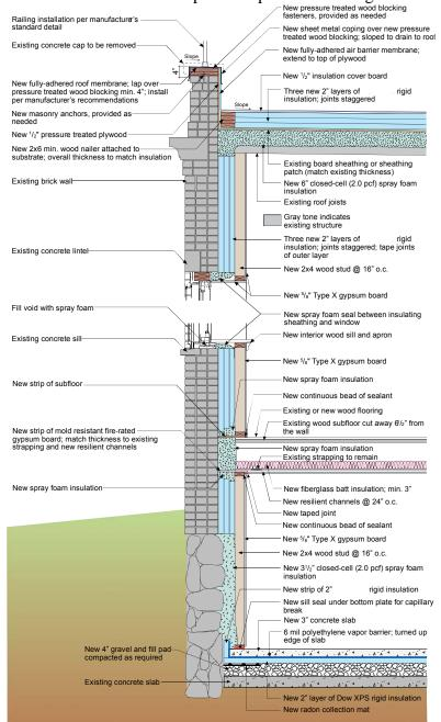
Figure 2: Bearing Masonry Interior Insulation Retrofit Approach
