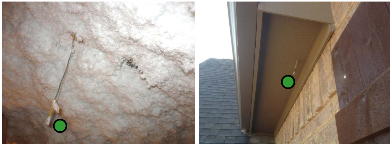
Figure 103: Interior attic temperature/RH sensor (L); exterior T/RH sensor under north soffit (R)
