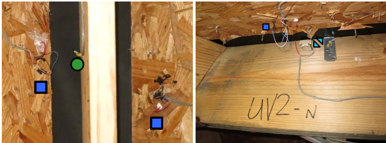
Figure 102: Ridge sheathing T/MCs and T/RH (L); ridge T/MC and wafer sensor (R)
