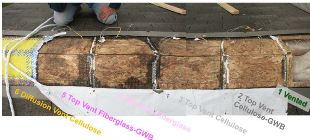
Figure 66: Ridge conditions, after removal of breather mesh
