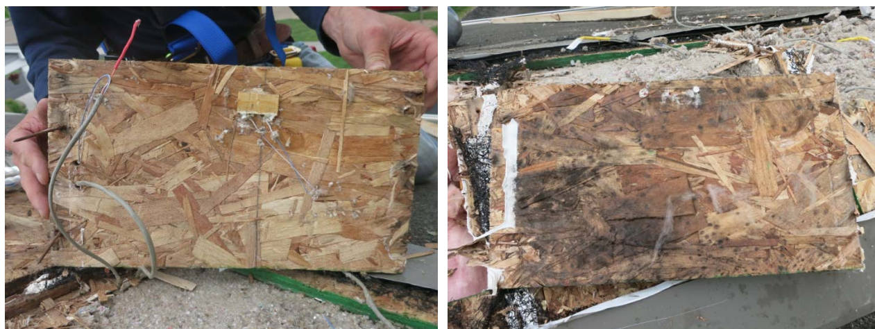
Figure 87: Top vent roofs, no interior GWB, East/front face; cellulose (L) and fiberglass (R)
