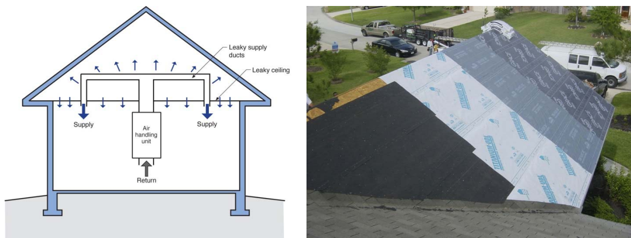
Figure 11: Air leakage communication from unvented attic to main space (L), and Houston-area roof underlayment study (R) (Lstiburek 2014)
