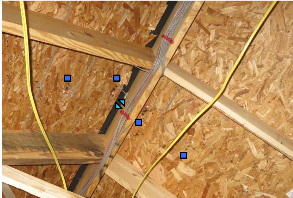
Figure 101: Typical ridge monitoring package, with sensors highlighted
