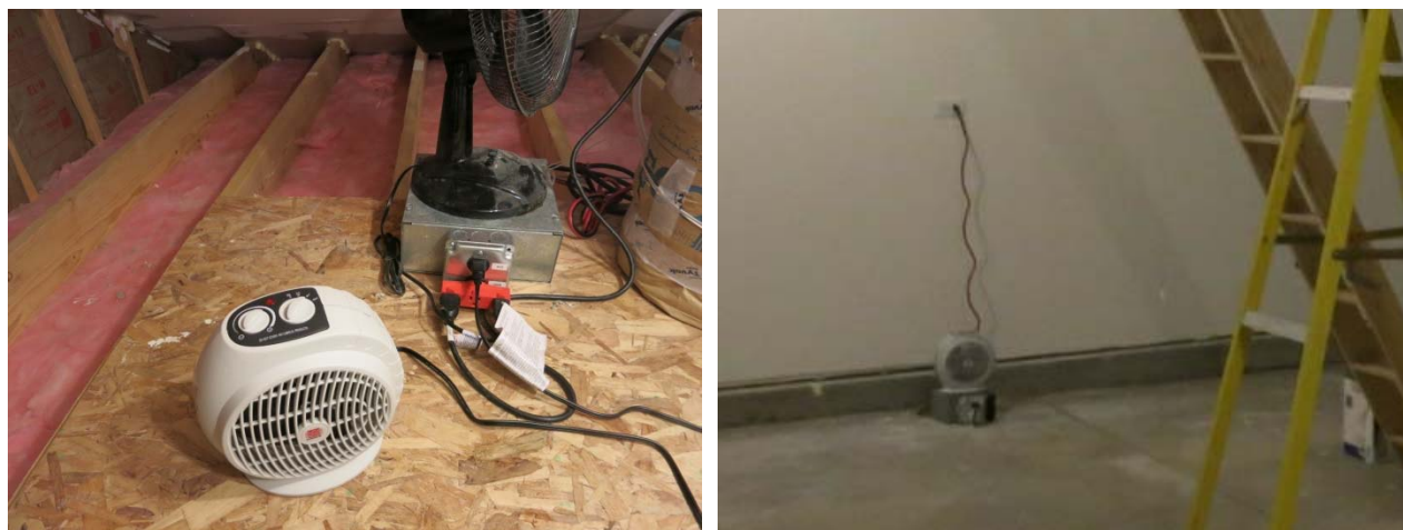
Figure 27: Experimental attic space heating (L), garage heating and relay box (right)
