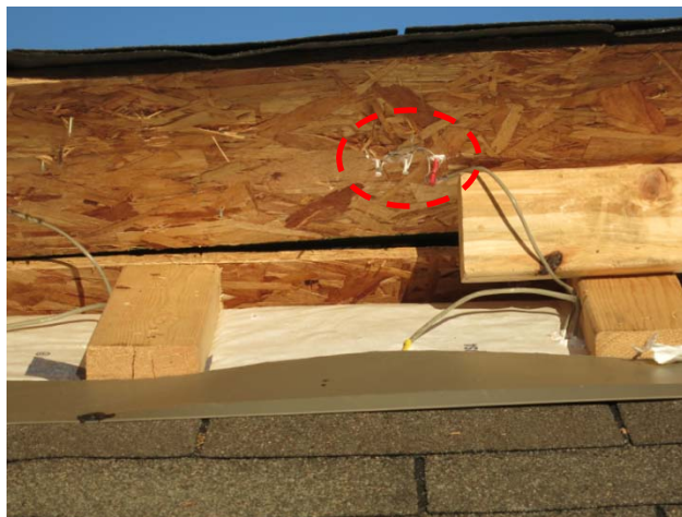
Figure 62: Roof “doghouse” sheathing moisture content sensor
