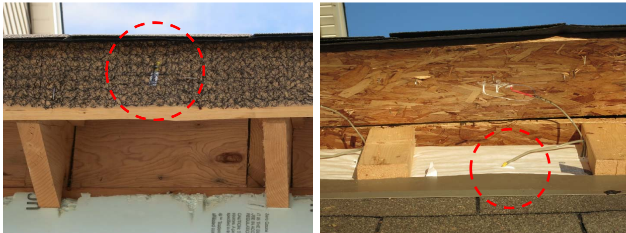
Figure 147: Intake (L) and exhaust (R) T/RH sensors for “top vent” roofs
