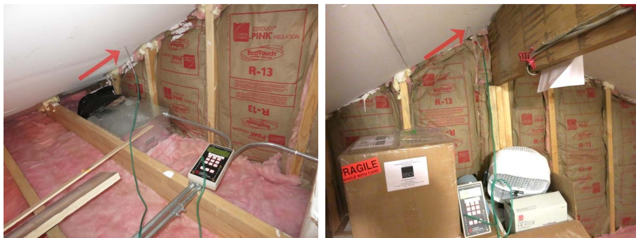
Figure 40: Testing pressure difference ( \Delta P ) across ceiling gypsum board in test attic
