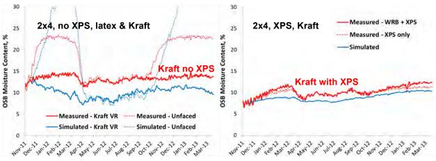
Figure 7: Measured vs. modeled OSB MC, 2x4 with/without XPS (Glass 2014)
