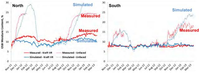
Figure 6: Measured vs. modeled OSB MC, 2x6 w. vinyl siding (Glass 2014)
