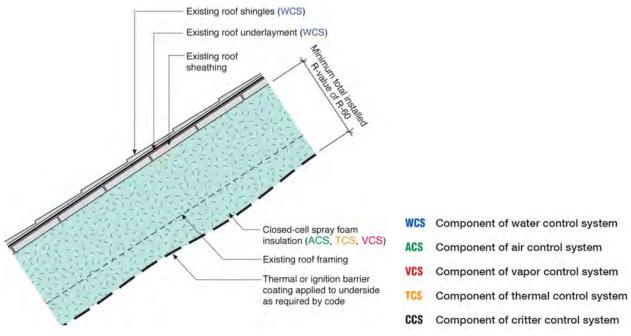
Figure 9: Identification of control layers in an assembly (BSC 2013)
