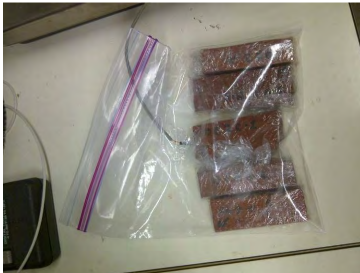
Figure 70: Thermistor installed within brick slice
