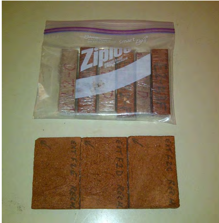
Figure 59: New (top) and old (bottom) brick slice samples
