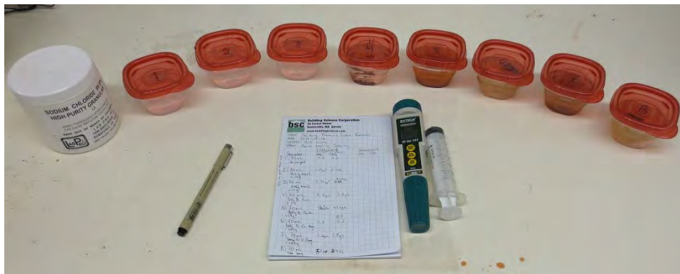
Figure 58: Preliminary masonry sample salinity testing, with deionized water control samples
