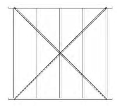
Figure 15. Diagonal strapping installed
