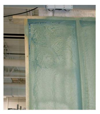
Figure 27. Stud flexure and ccSPF tearing
