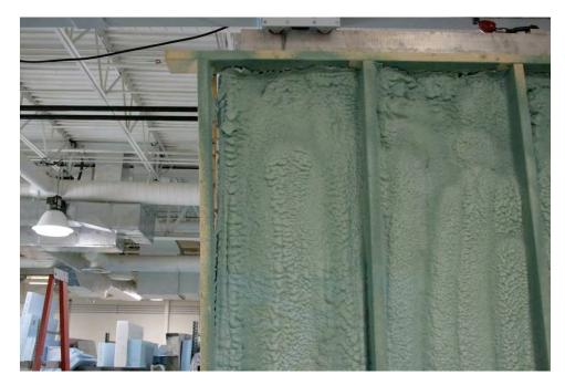
Figure 30. ccSPF tear propagation
