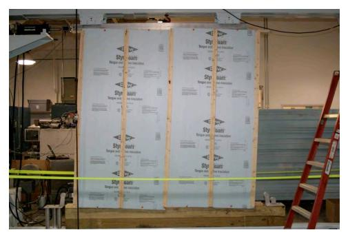
Figure 24. XPS sheets twisted in-plane
