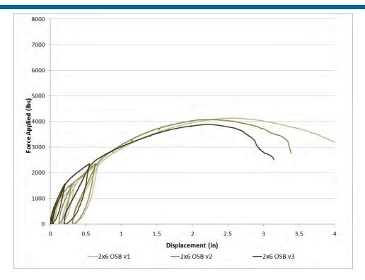
Figure 18. Standard OSB wall results
