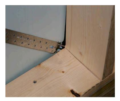
Figure 22. Metal strap nail pullout
