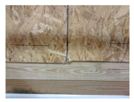
Figure 19. OSB failure at fastener
