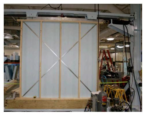
Figure 20. Structural test wall 1 installed in apparatus
