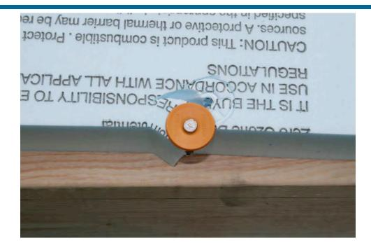
Figure 23. Nail pulling through XPS
