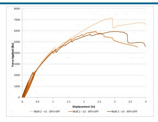
Figure 26. Structural test wall 2 results
