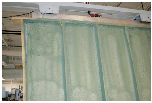
Figure 28. ccSPF tear propagation
