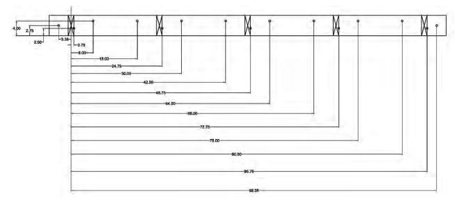
Figure 13. Bottom plate screw pattern
