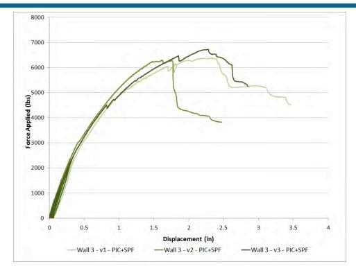
Figure 29. Structural test wall 3 results
