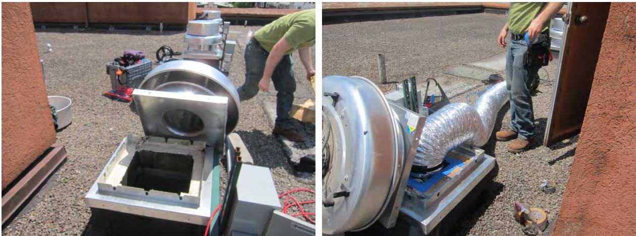
**Figure 72. Duct leakage testing of EF-3 (post-retrofit)**
