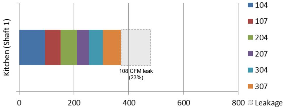
**Figure 41. Unit airflows compared to rooftop fan airflow, EF-1 (kitchens)**
