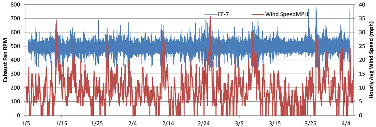
**Figure 82. EF-7 fan speeds with hourly exterior wind speeds for KPHL weather station**
