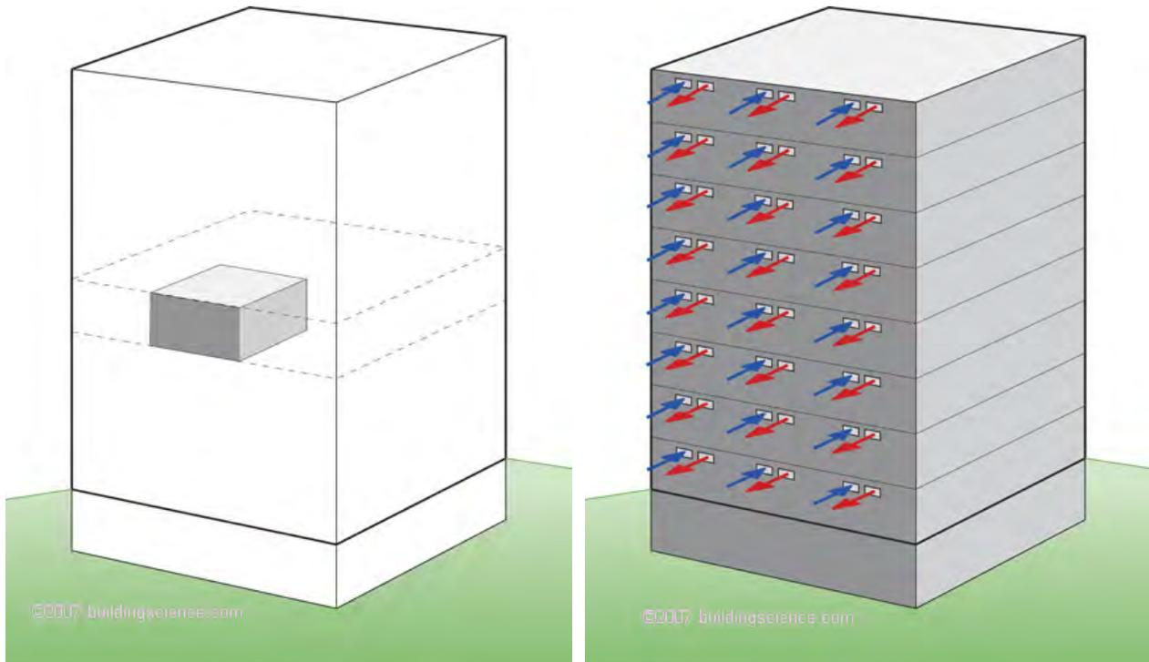
**Figure 5. Ideal unit compartmentalization (L) and individual unit ventilation supply/exhaust (R)**
