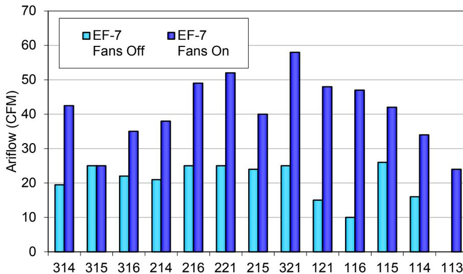
**Figure 65. EF-7 airflow measurement of individual unit exhaust fans, turning unit fans on**
