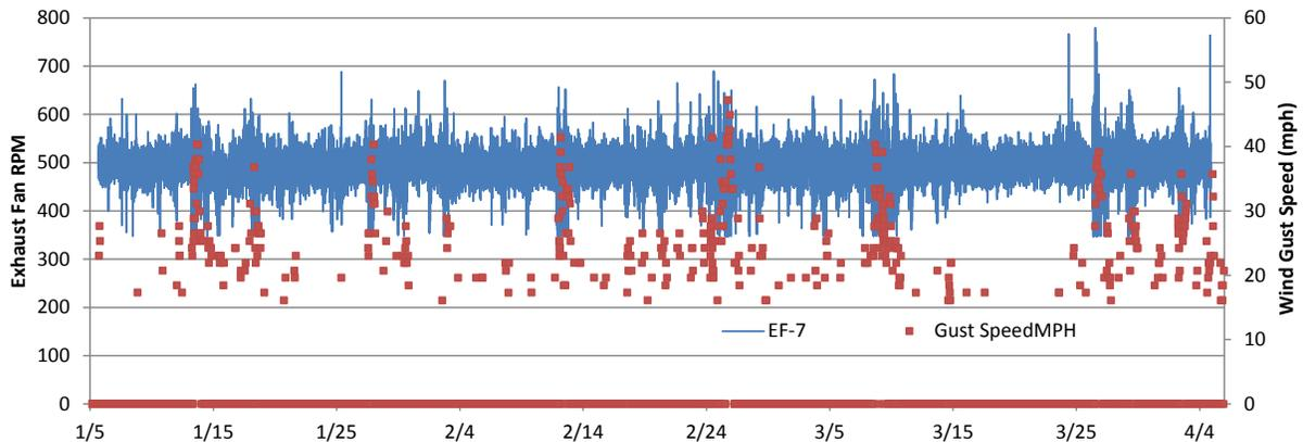
**Figure 83. EF-7 fan speeds with wind gust speeds for KPHL weather station**
