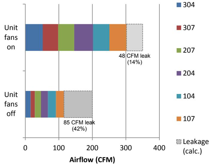
**Figure 68. EF-1 unit airflows and rooftop fan airflow (calculated duct leakage), turning unit fans off**
