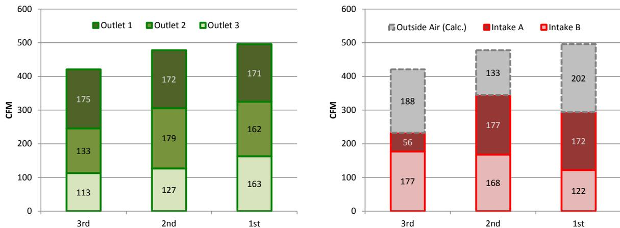
**Figure 91. Ventilation outlet (L) and intake (R) flow measurements, with calculated outside air**
