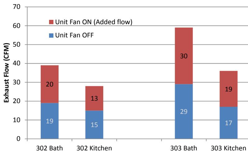
**Figure 76. Unit exhaust airflows with unit fan turned on and off**
