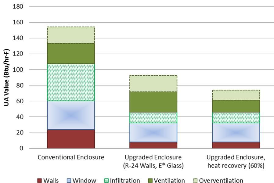
**Figure 7. Relative contributions of opaque wall, glazing, ventilation, and infiltration (UA values)**
