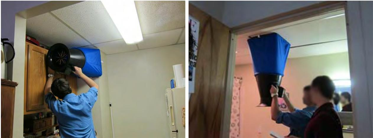
Figure 37. Airflow testing of unit exhausts with flow capture hood; kitchen (L) and bath (R)
