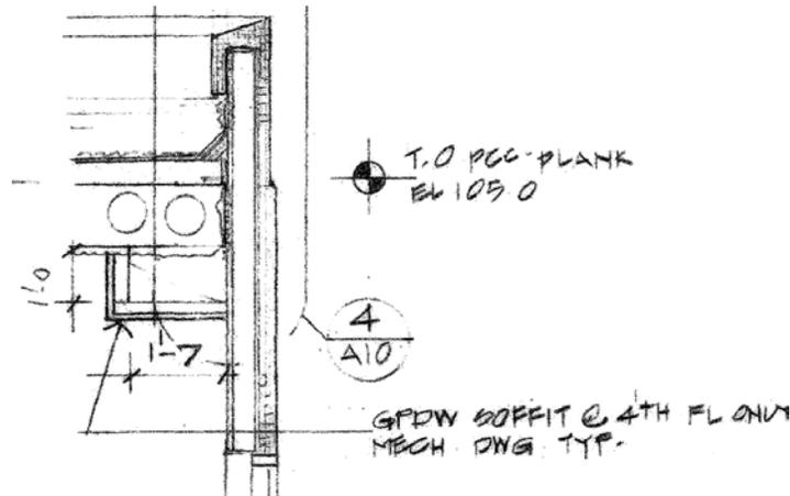
**Figure 46. Top floor mechanical soffit and parapet detail (Section A10.10)**
