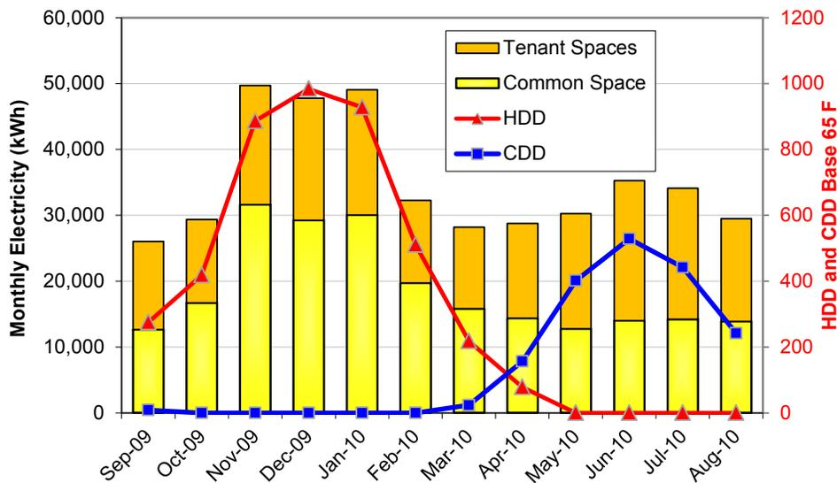
**Figure 13. Pre-retrofit energy performance (common + tenant) electricity use, with HDD/CDD**
