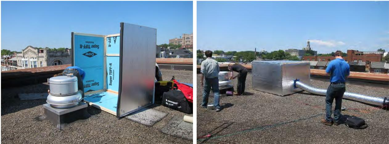
**Figure 34. Powered flow capture enclosure for rooftop exhaust fans showing construction**
