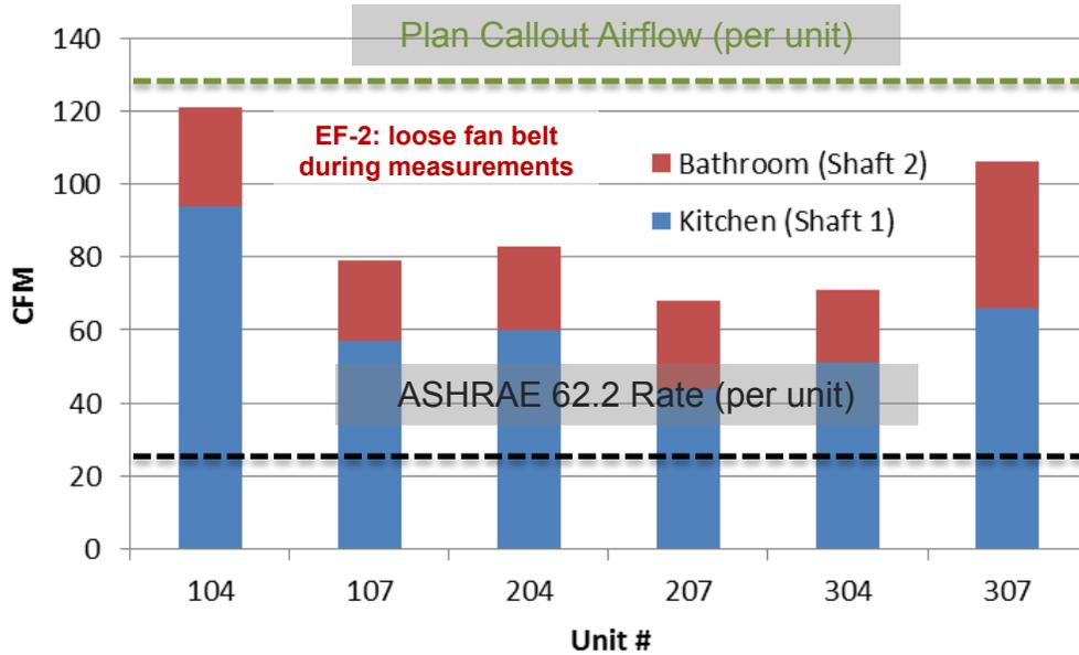
**Figure 39. Unit airflows for bathroom and kitchen exhaust fans, shafts 1 and 2**
