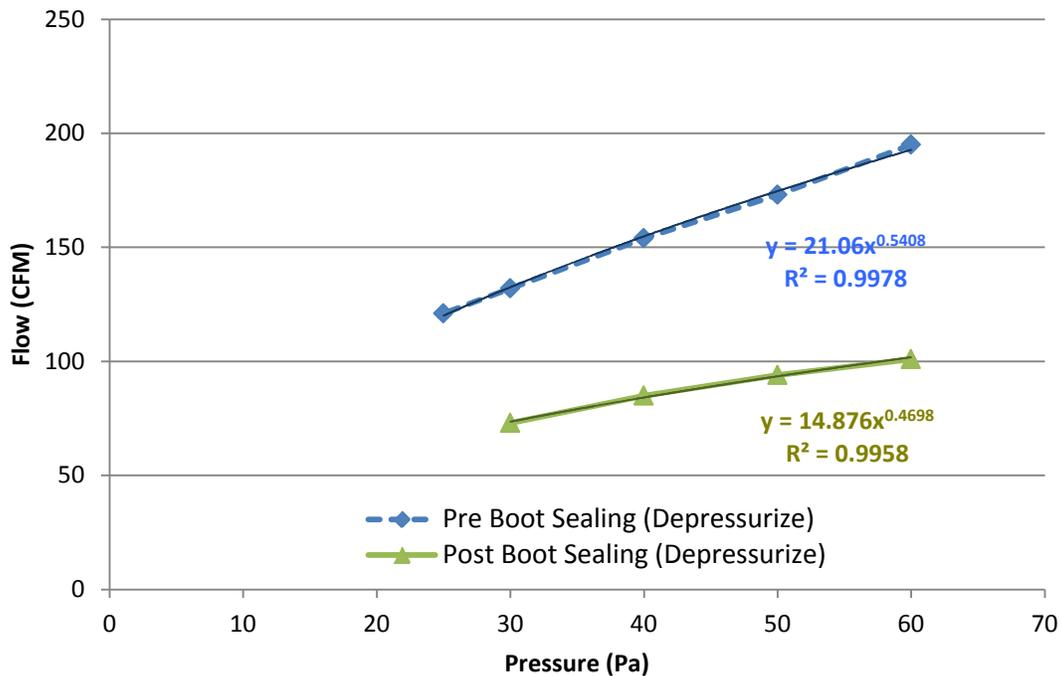
**Figure 32. Multipoint air leakage data for EF-1 with pre- and post-register boot sealing**
