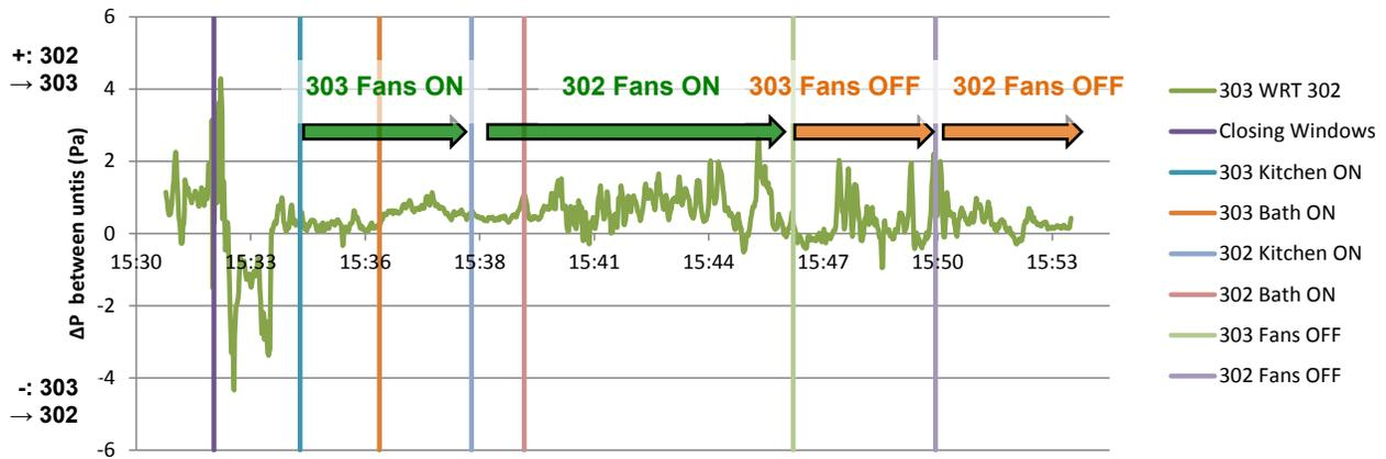
**Figure 75. Interunit pressure difference measurement**
