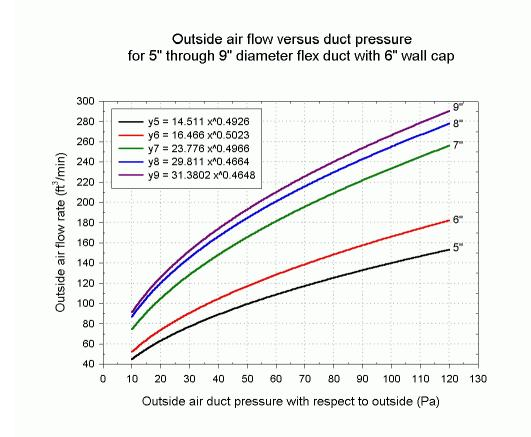
Duct static pressure should be measured in the duct, outboard (i.e., on the outdoors side) of the filter and damper (if installed). Also, although the graph uses "outside air duct pressure with respect to outside," the indoor-outdoor pressure difference should not be large in our Building America houses (~1-2 Pa, at most). Therefore, measuring the outside air duct pressure WRT indoors should work. Of course, if you are working in a vented attic, it is essentially at outside pressure.
