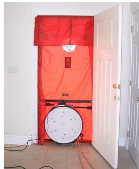
Both results greatly surpass the targets of 40 CFM duct leakage to outside and 80 CFM total duct leakage. In addition to the Duct Blaster® and blower door tests, room by room air flows were tested using a flow hood and all found to be as designed.
