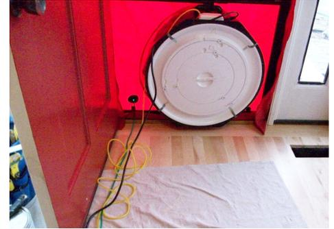
as the overall increased surface area and volume due to the addition and the restructured roof. The post-retrofit measurement is roughly equivalent to 1.7 ACH 50 when using the air barrier boundary to establish the volume.
