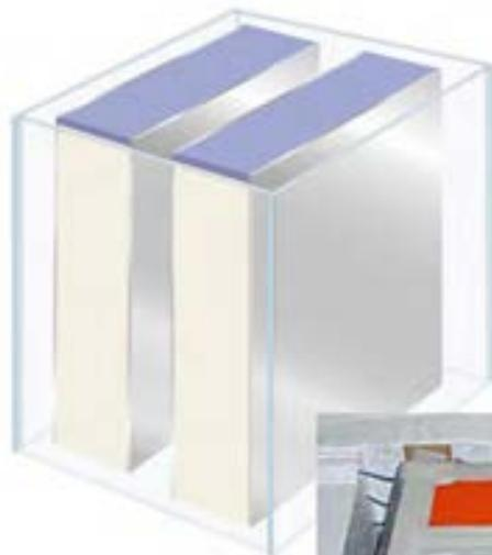
Figure 70: Holding chamber for replicas. **BELOW**, finished chamber with cover, with replicas in place. The chamber is insulated from changing ambient temperatures by a polystyrene foam outer box.
