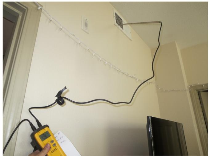
Figure 14: Measuring “split” at supply
