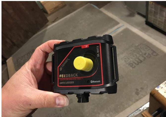
**Figure 3:** Tramex DL-RHTX T/RH meter
