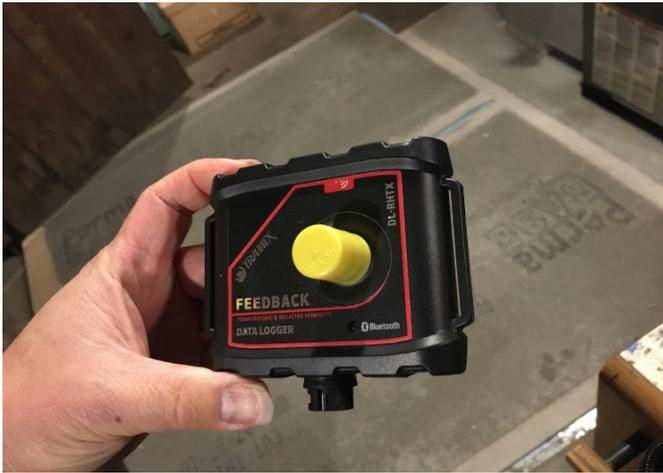
Figure 3: Tramex DL-RHTX T/RH meter
