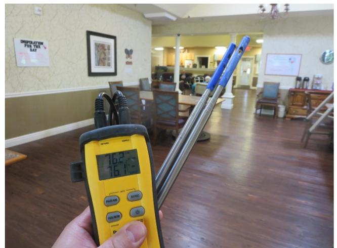
Figure 2: Dual in-duct psychrometer
