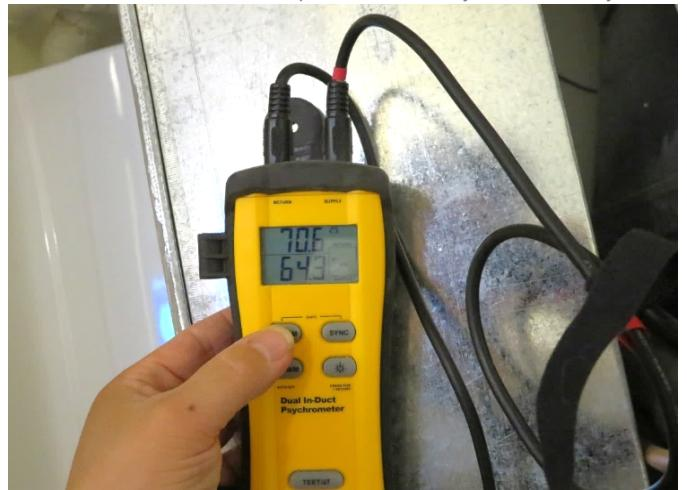
**Figure 13:** Measuring “split” across an AHU
