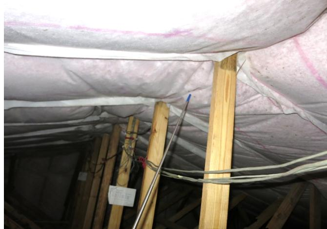
**Figure 10:** Measuring T and DP stratification
