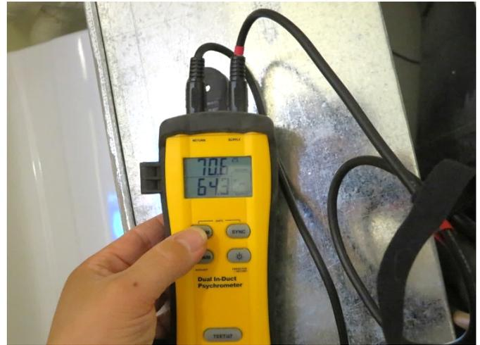
Figure 13: Measuring “split” across an AHU
