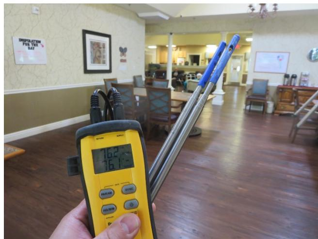
**Figure 2:** Dual in-duct psychrometer
