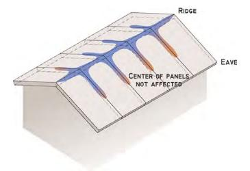
Figure 3: Ridge Rot – The failures were concentrated at ridge locations. Air leakage from the interior carried moisture laden air to cold surfaces where it accumulated and led to damage.
