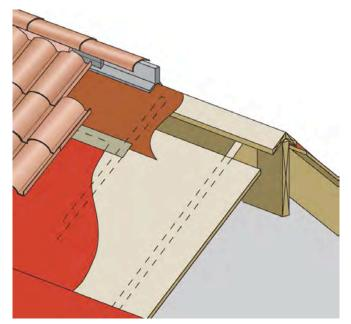
**Figure 6: Vapor Diffusion Vent for Tiles**—Works with tiles too—it's the same slot used for typical vented roofs, except covered with vapor open membrane.
