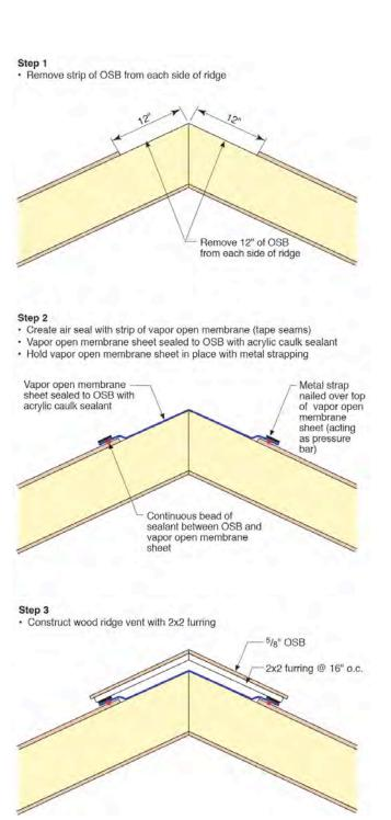
**Figure 4: Vapor Diffusion Vent** – Not a vent for airflow. No airflow. Just vapor flow in the form of vapor diffusion. We and others have been fixing SIP roofs – and other roofs - all over using this approach.
