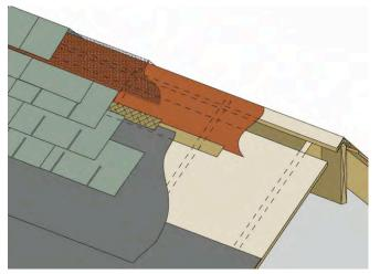
**Figure 5: Vapor Diffusion Vent for Shingles**—Any off-theshelf ridge vent works. The only change is covering the vent area cut through the sheathing with a water tight but vapor open covering. A high perm "housewrap" works – over 20 perms. A high perm exterior sheathing such as fiberglass faced gypsum board also works as a vapor open covering.
