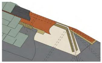
**Figure 7: Vapor Diffusion Vent for Hips**— Just need the upper 4 feet of the hip to be diffusion vented.
