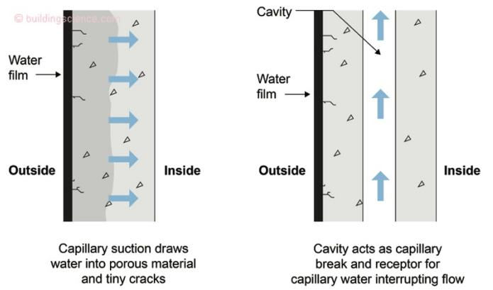
Figure 3: Capillarity – A driving force for rain entry.
