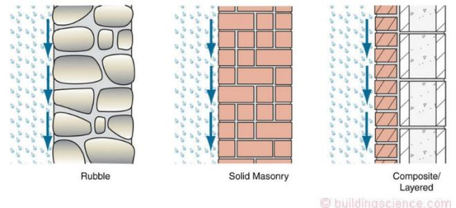
**Figure 8: Mass/Storage -** Rainwater entry controlled by providing materials that can store, absorb, redistribute and dry (Courtesy of Straube, 2012).
