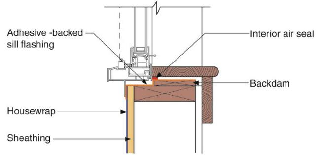
A strip of wood nailed at the back of the rough opening sill forms a dam to prevent water from draining into the interior.
