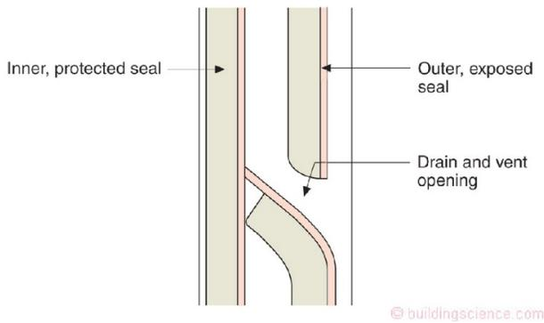
**Figure 12:** Two-Stage Joint Section - Section through a two-stage joint that uses sealant to direct water to the exterior.
