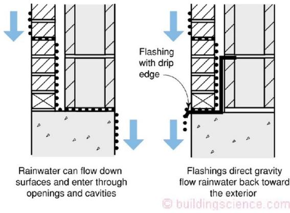
Figure 1: Gravity – A driving force for rain entry.
