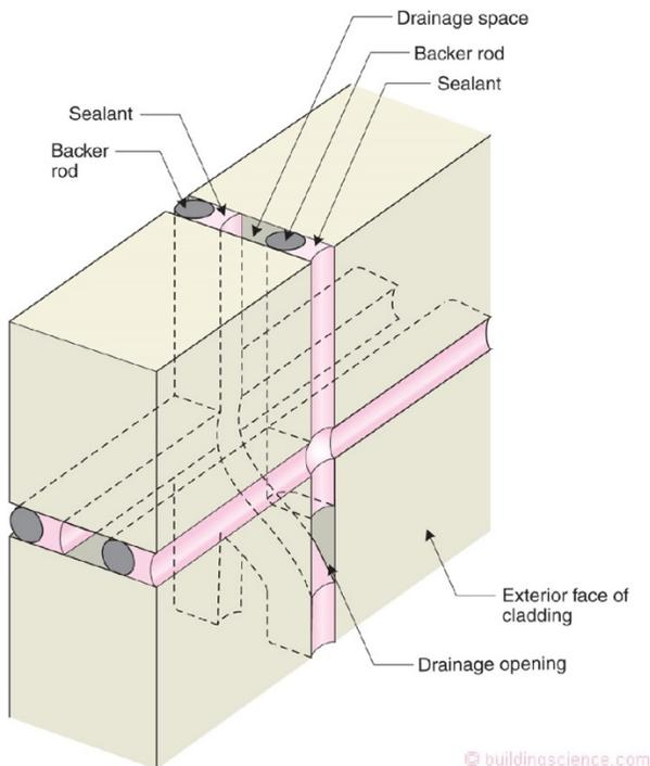
**Figure 13:** Three Dimensional Detail of Two-Stage Joint - Drainage paths are shown. The outer seal is exposed to the elements – ultra violet light, heat and water – but the assembly still works because of the interior protected seal.
