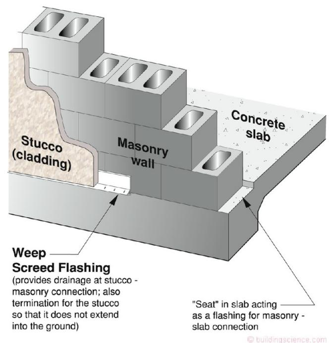
**Figure 10:** Mass/Storage Assemblies – Mass/storage assemblies store, absorb, redistribute and dry rainwater and groundwater without being damaged such as a masonry wall rendered with a Portland cement based stucco.
