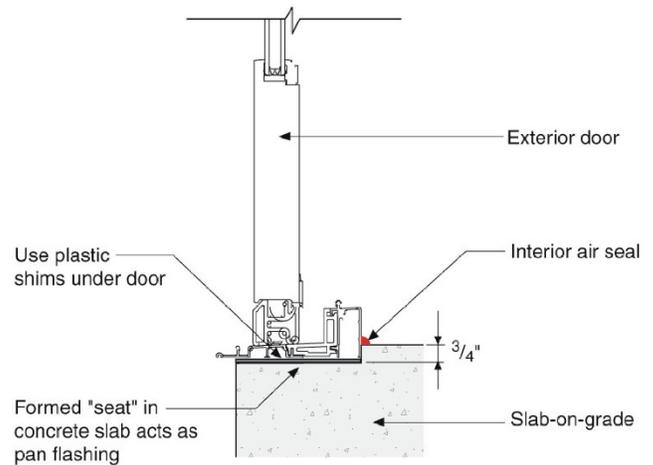
Forming a depression in a cast-in-place floor slab creates a built-in drainage pan for mulled entry doors and sliders, which are prone to leakage at joints.
