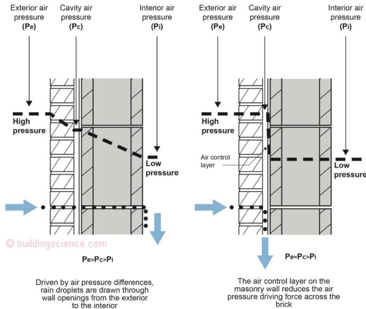
Figure 5: Air Pressure – A driving force for rain entry.
