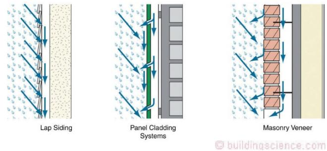
**Figure 6:** Drained – Rainwater entry controlled by providing drainage (Courtesy of Straube, 2012).
