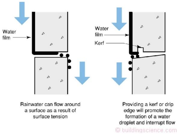
Figure 2: Surface Tension – A driving force for rain entry.
