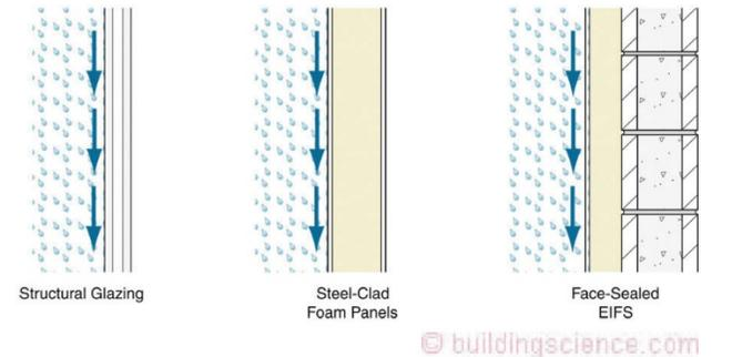
**Figure 7:** Barrier - Rainwater entry prevented by providing a barrier (Courtesy of Straube, 2012).
