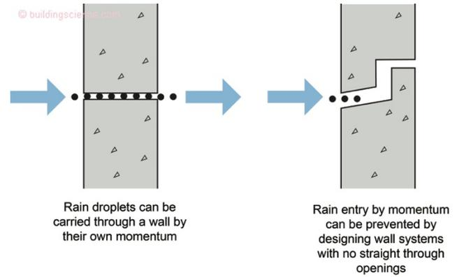
Figure 4: Momentum - A driving force for rain entry.
