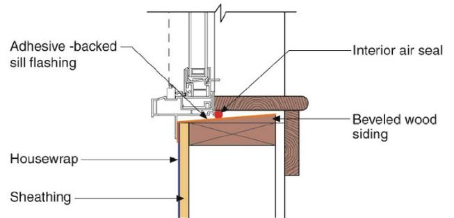
A piece of wood bevel siding nailed over the sill to create positive drainage toward the exterior is even better. Note that the rough opening needs to be enlarged to account for this and tapered shims in the opposite direction of the slope may be required.
