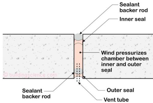
**Figure 11:** Two-Stage Joint – Continuous inner seal and a drained and vented cavity between the continuous inner seal and a weeped outer seal.
