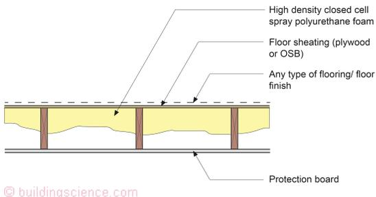
**Figure 13:** Vented crawlspaces must keep air and vapor out of the crawlspace floor framing. Only high density closed cell spray polyurethane foam should be used in all IECC Climate Zones.
