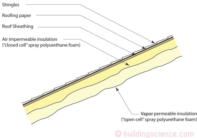
**Figure 6:** Hybrid attics can be constructed using a combination of high density closed cell spray foam and low-density open cell spray foam.
