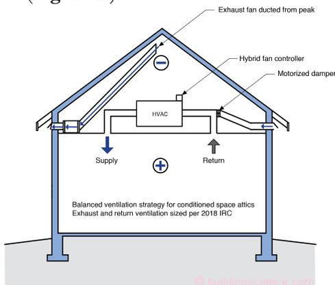
**Figure 10:** The best way to remove moisture from the attic space is to provide air change. Air is exhausted from the peak of the attic using an exhaust fan ducted to the exterior.
