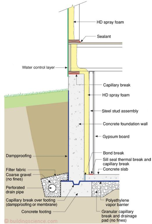
**Figure 11:** Spray foam insulation can be directly applied to the interior of concrete foundation walls.
