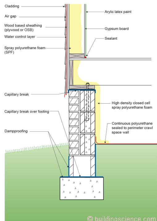
**Figure 15:** Conditioned crawlspaces should be constructed as “mini” basements and completely connected to the house.
