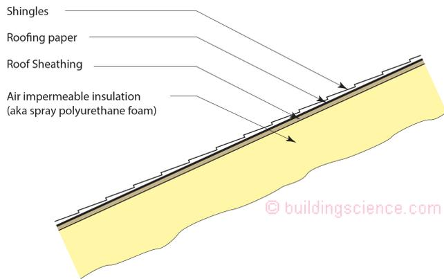
**Figure 5:** Unvented conditioned attics can be constructed by installing low density open cell or high density closed cell spray foam directly to the underside of the roof deck.
