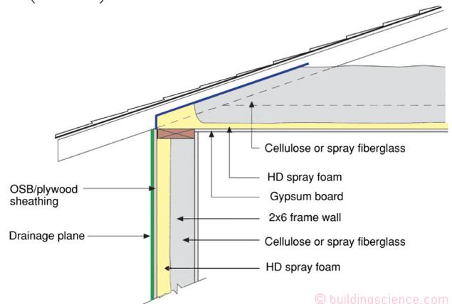
**Figure 8:** Vented unconditioned attics are typically constructed using spray foam in conjunction with fiberglass or cellulose insulation. The key to the performance of vented unconditioned attics is continuity of the air control layer located at the ceiling plane.
