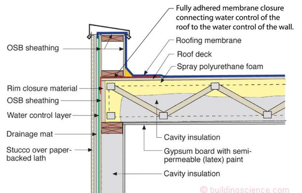
**Figure 9:** Most low slope roof construction using spray foam use a hybrid approach where a combination of high density closed cell spray foam is used with fiberglass or cellulose insulation.
