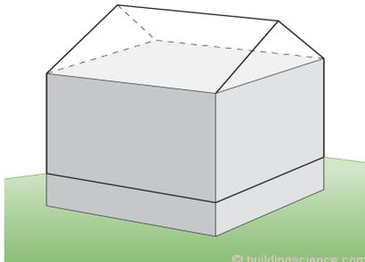
**Figure 1:** Houses have walls, roofs and foundations that each have to be connected to each other providing continuity of the water control layer, air control layer, vapor control layer and thermal control layer.
