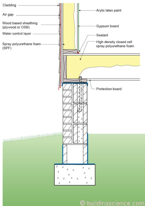
**Figure 14:** A protection board such as fiber cement should be installed to prevent animals from getting into the floor assembly.
