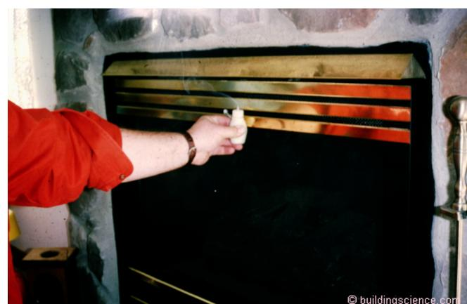
**Photograph 5: Backdrafting Gas Fireplace** - Soot from standing pilot lights on gas fireplaces are a big source of particulates. When the full burners are on venting occurs. When only the pilot light is on backdrafting is common.
