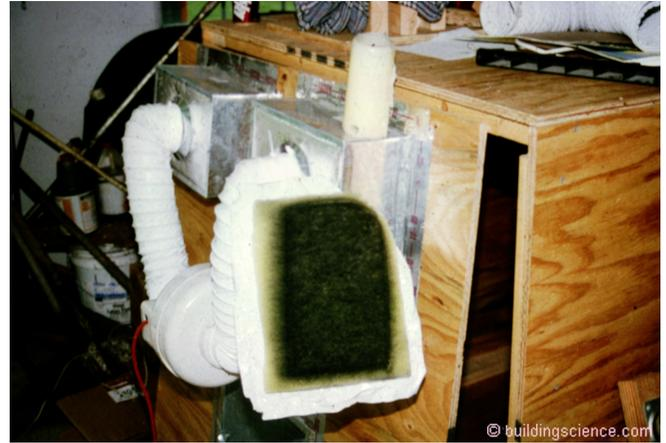
**Photograph 4: Environmental Chamber Test** - Who would have thought that candles could cause so much damage and generate so much soot. A wonderful “bench top” experiment by an old school engineer shows the amount of soot from a 30 minute candle burn.
