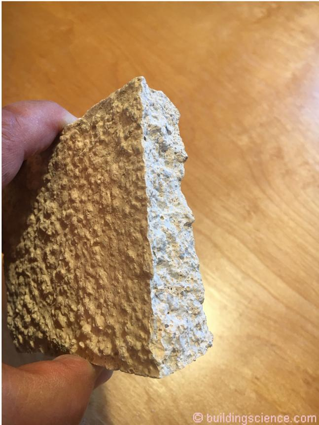
**Photograph 9 – Coating on Back of Manufactured Stone Veneer:** Manufactured stone is back-coated (“sealed”) to prevent excessive water absorption out of the thin set. The issue is desiccation of the polymer modified thin set mortar leading to not establishing a bond. So a “porous” not real stone is made to behave like a non-porous real stone with the back-coating.
