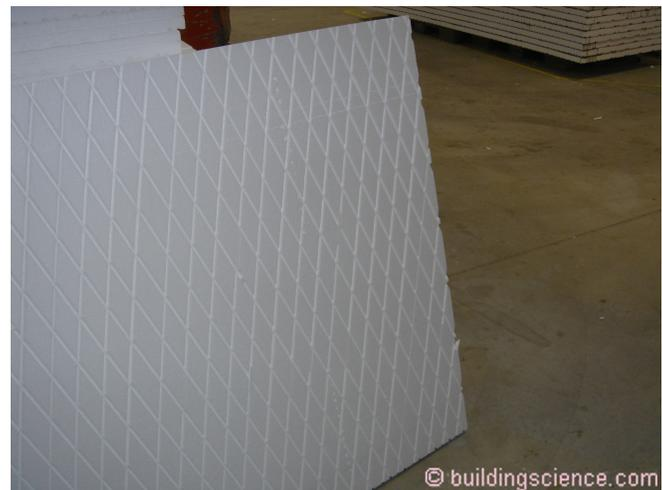
**Photograph 6: Drainage Grooves** – Channels cut into the back of expanded polystyrene (EPS) to provide drainage. This comes to us from New Zealand. Apparently the Kiwis have heard of Vitruvius.
