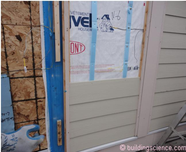
**Photograph 4: Hygric Redistribution** – Test hut experiment measuring hygric redistribution under various air spaces, cladding types, sheathing types and thermal resistance levels. In this image the air gap is 3/8 inch coupled with fibercement siding, a high perm housewrap and OSB sheathing.
