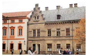
**Photograph 2: Prague, Czech Republic**—The house on the right is brick masonry. The house on the left is stucco over brick masonry. As brick and stone buildings get old they leak. So how do we handle it? We try repointing the brick first. Then we paint over the brick. And then at the end we stucco over the brick. We do this all over the world. As buildings age we repoint them, paint them and then stucco them.
