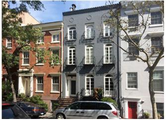
**Photograph 1: "Aging Gracefully"**—Manhattan, Soho, right down town. What's so interesting about this streetscape? The house on the left is brick masonry. The house in the middle is painted brick masonry. The house on the right is stucco over brick masonry. Better and better water control from left to right. Owners figure things out.
