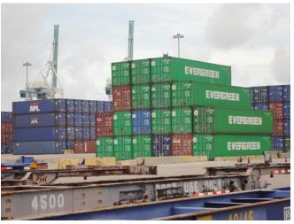
**Photograph 3: Stack Effect** – A different kind of stack effect for sure. Each box has strong corner posts so that they can be stacked.
