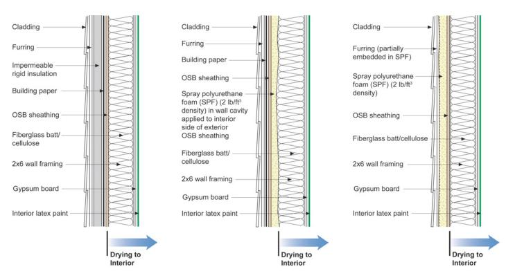
Figure 3a (above *left*): High Performance Exterior Continuous Insulation Sheathing – This wall works everywhere. The thermal resistance of the exterior continuous insulation is climate dependent. Figure 3b (above *middle*): Cavity Foam Wall – This wall works everywhere. The thermal resistance of the SPF in the cavity is climate dependent. Figure 3c (above *right*): High Performance Exterior Spray Foam Wall – This wall works everywhere. The thermal resistance of the SPF is climate dependent.
