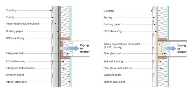
Figure 4a (above left): Exterior Insulated Rim Joist – The thermal resistance of the exterior continuous insulation is climate dependent. Figure 4b (above right): Spray Polyurethane Foam Rim Joist - The thermal resistance of the SPF is climate dependent.
