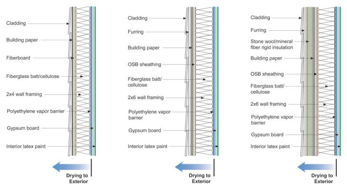
Figure 2a (above *left*): The "Old Plastic Wall" – The wall that kinda worked with fiberboard but not with OSB. Don't use this wall with air-conditioning. Figure 2b (*above middle*): The "New Plastic Wall" – The wall that works with OSB because of the ventilated cladding. Don't use this wall with air-conditioning. Figure 2c (*above right*): High Performance Plastic Wall – This wall works well. Just don't use it with air-conditioning.
