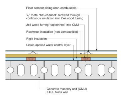
**Figure 5: CMU Wall**—Wood 2x4's on the flat are tappconned into the masonry to provide a structural transition for the cladding attachment. A liquid applied water and air control layer is applied directly to the masonry prior to the installation of the 2x4's. Rigid insulation is installed between the 2x4 furring and then a continuous layer of rockwool is installed. The exterior fibercement cladding is installed as before.
