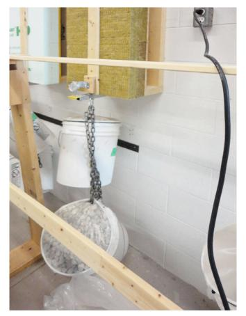
**Photograph 2: Stress Test**—How do you stress the assemblies? Fill 5-gallon plastic pails with rocks and hang them from the assemblies. And wait. And wait. And still wait. You have to wait a long time. This "creep" thing might creep up on you and you don't want to be surprised. Surprises are bad if you are an engineer.
