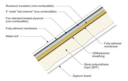
**Figure 2: Non-Combustible Vented Roof With SPF**—One layer of rockwool rigid board insulation provides the fire protection on the top side of the structural roof deck. The spray polyurethane foam (SPF) handles the condensation control. Note that in IECC Climate Zones 5 and higher the SPF must be 2 lb/ft<sup>3</sup> density. Same comment as for Figure 1 - the metal "hat-channel" can be replaced with fire retardant treated wood 2x4's lying "flat."
