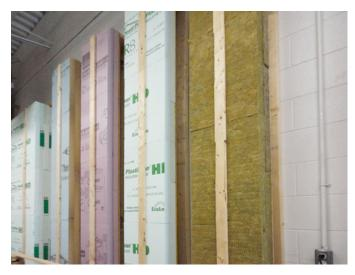
**Photograph 1: Build Stuff and Break It**—The only way to know is to test it to failure and then you know. How do you figure out how to attach cladding through various types of rigid insulation? You build a whole bunch of assemblies and see. There is no other way.
