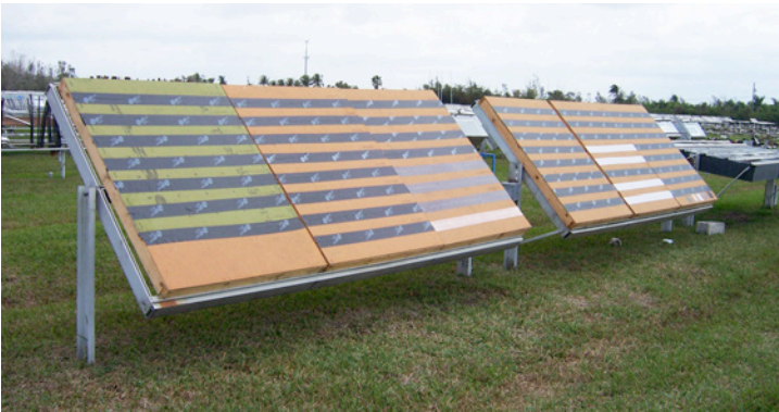
Photograph 12: Proprietary Florida Exposure Test Site - Not one of our sites. Lots of folks are testing things this way. Especially the folks who make things to sell. Nothing beats real world exposure.
