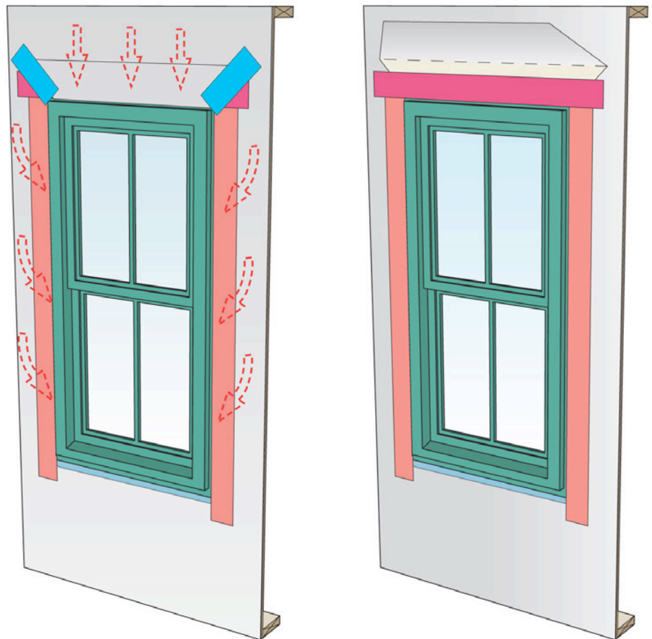
Figure 1: Water Entry at Window Opening (left) – It is important to address water running behind building wraps and housewraps at window heads and the sides of window openings. Figure 2: Control of Water at Window Head (right) – The top window flange is taped directly to the sheathing with “flashing tape.” Note how the building wrap or housewrap is cut and folded upwards to expose the sheathing so that the “flashing tape” can be installed. Once the tape is installed, the flap is folded back down. This works exceptionally well.
