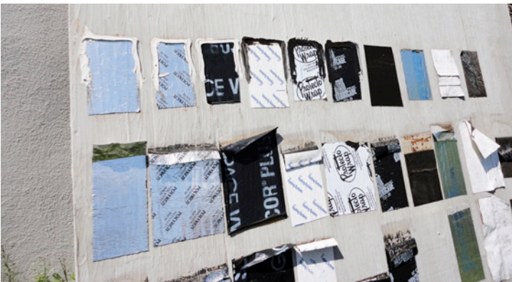
Photograph 13: Horizon Homes Test Panel – You would be surprised at the number of homebuilders who are testing the stuff they plan to use to see how it works. Our rule-of-thumb is that if it works exposed like this for 2 years you are pretty much good to go.
