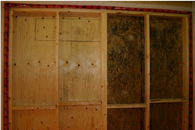
**Photograph 2 – OSB versus Plywood:** At the University of Waterloo “skunkworks” an OSB panel and plywood panel are exposed to identical temperature and humidity conditions over the same time period – the panels were side by side in a climate chamber. The OSB is covered with mold – the plywood is pristine. OSB needs to be used differently than plywood – it needs to be protected differently than plywood.
