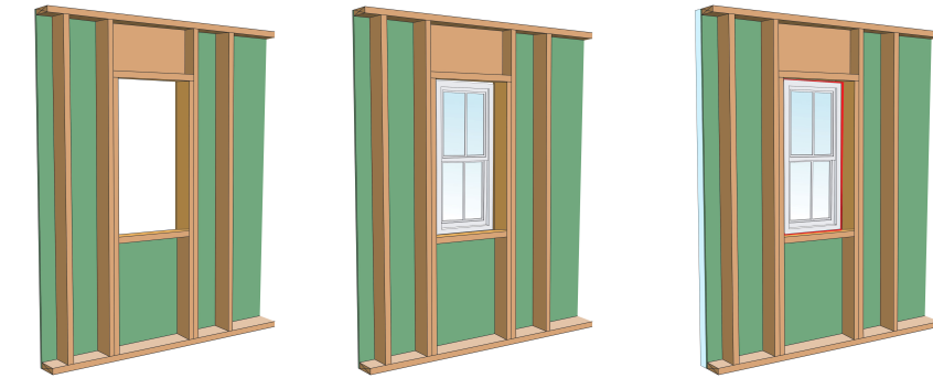
Figure 1 – Window Installation Sequence For “Bump Outs” And Foam Sheathing. The water and air control layer is the sheathing behind the continuous insulation. Note the “bump out” at the perimeter of the rough opening. Note the sloping sill. Note that the pan flashing can be liquid applied or a formable membrane. Note that the seams in the continuous insulation do not need to be sealed or taped.
