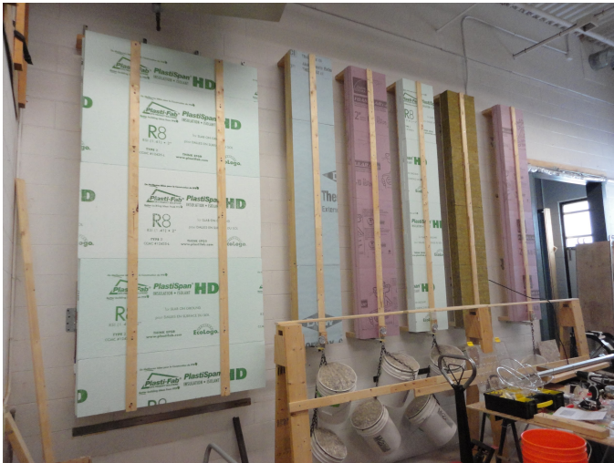
Photograph 4 – Creep Testing - We have hung things off of foam sheathing to figure out long term creep performance.
