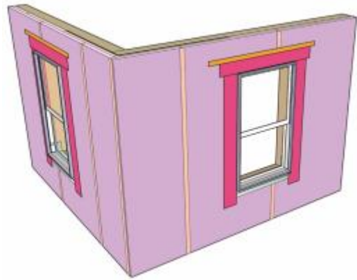
Figure 4a: Continuous Exterior Insulation – Water control layer is the exterior face of the insulation. Note the taped joints.
