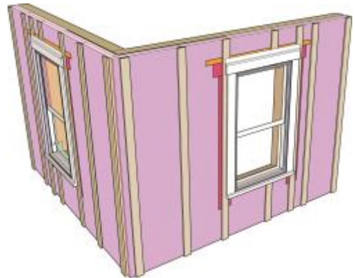
Figure 4c: Window Trim Installed – Note that the flashing above the horizontal trim at the top of the window is installed to protect the trim not to protect the window unit.
