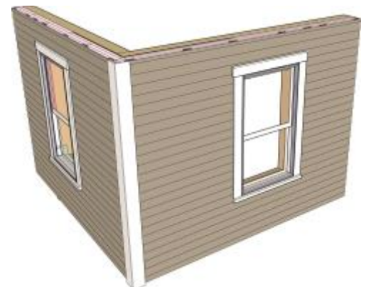
Figure 4e: Cladding Installed – Sealed on all six sides over an air gap. Awesome.
