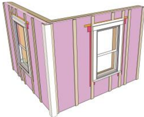
Figure 4d: Corner Trim Installed – The two corner trim pieces are attached “to themselves” and then the “L-shaped” trim assembly is attached to the gapped wood furring at the corner.
