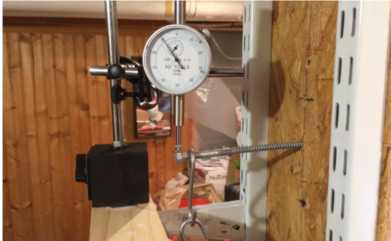
Figure 6. Simple cantilever screw bending test
