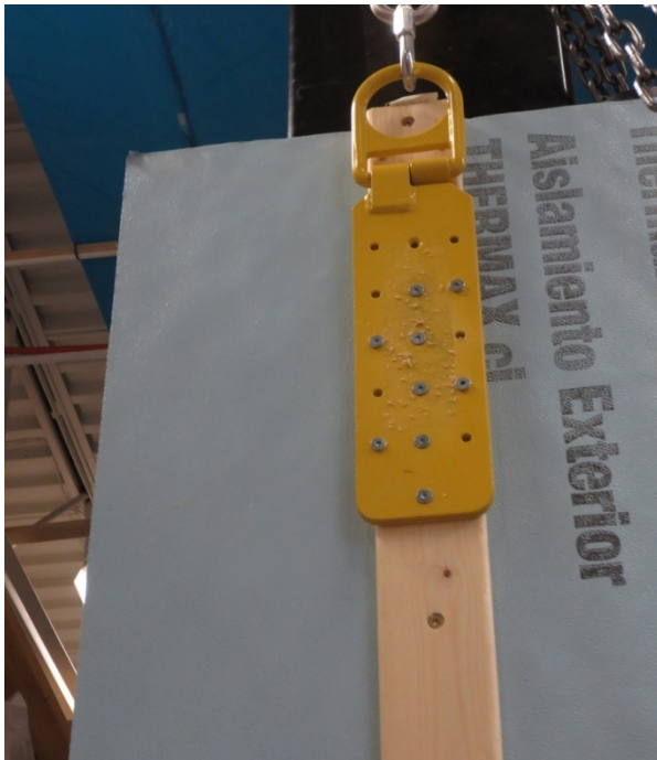
Figure 19. 5000-lb anchor at top of furring strip
