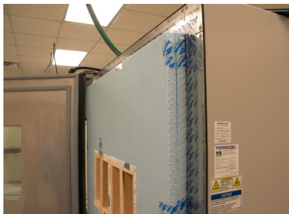
Figure 16. Assemblies installed in climate chamber opening
