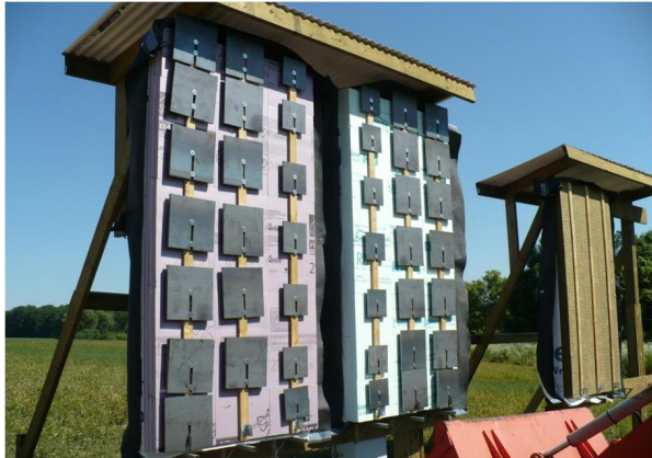
Figure 21. Exposed wall assemblies loaded to representative cladding weights
