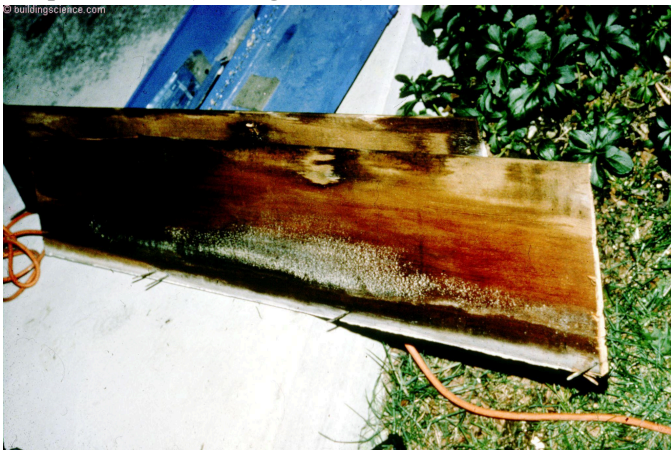
Photograph 4: Rotting moldy siding -thank you CHIP
