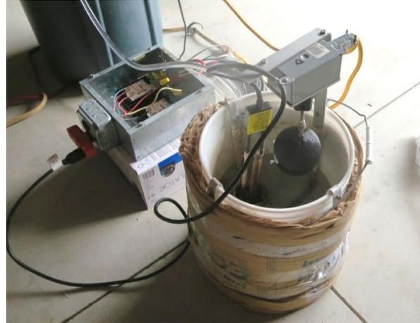
Figure 125. Humidifier bucket, heater, and float switch
