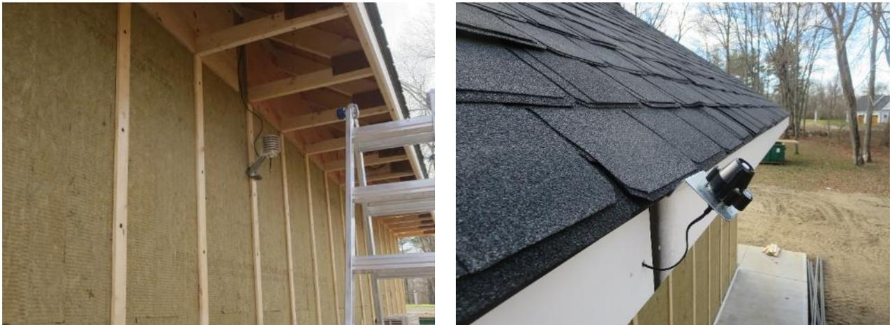
Figure 34. Exterior temperature/RH sensor (left), roof solar radiation sensor (right)
