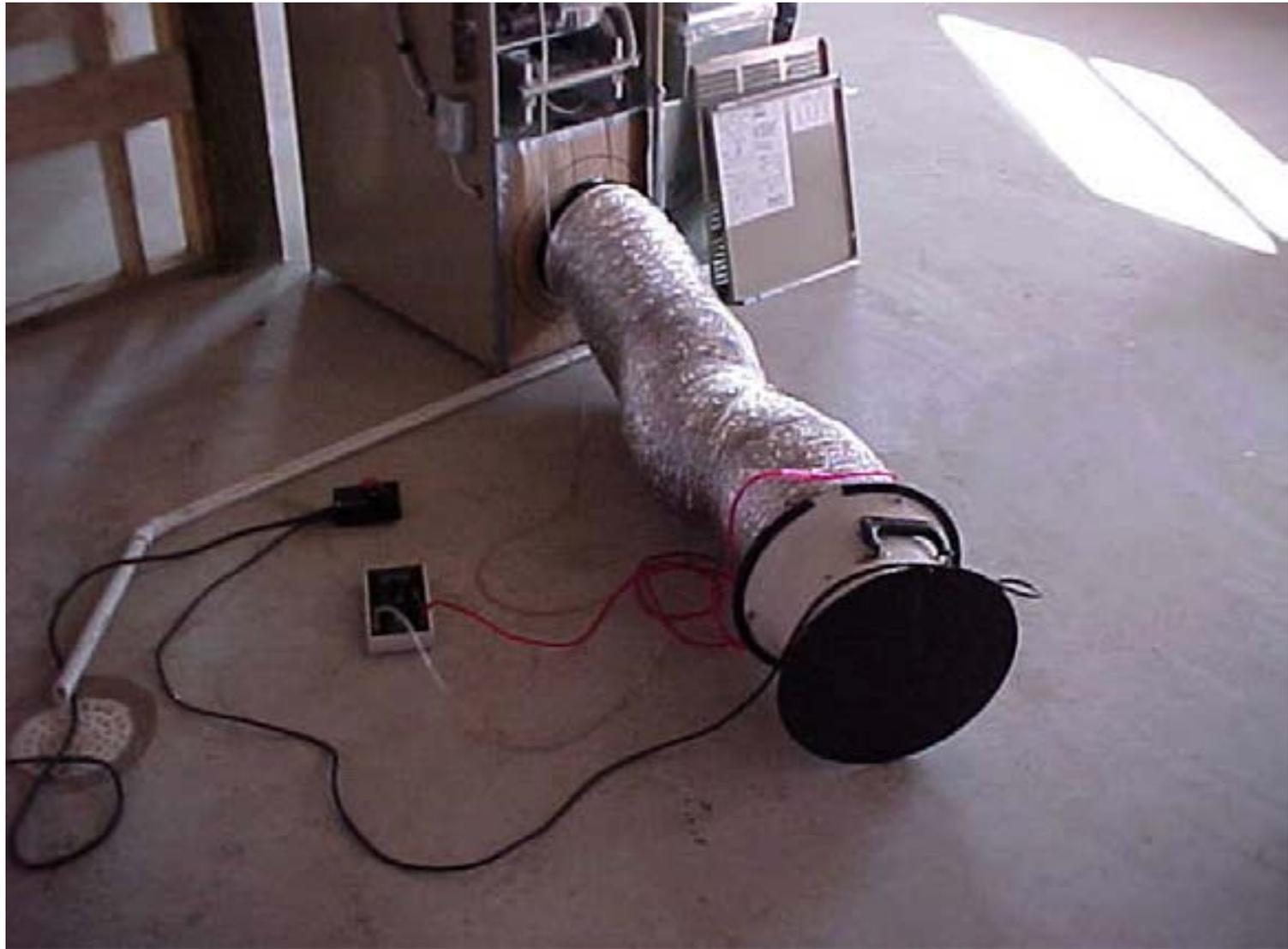
Duct Leakage Should Be Less Than 5% of Rated Flow As Tested By Pressurization To 25 Pascals
