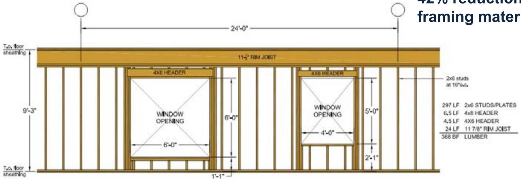
**Exterior Wall Framing Elevation (Typical Design)**
