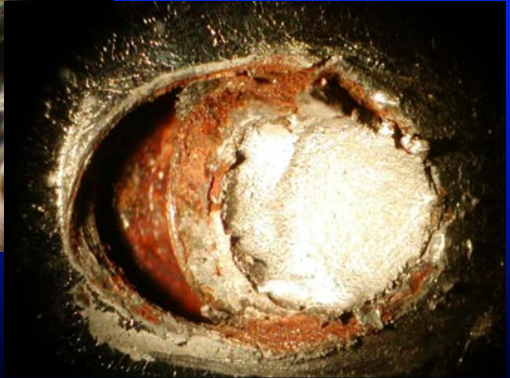
Failed Connection – 1537 Cycles
